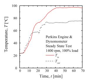
Figure 6. Preliminary steady state test with a Perkins Engine.
