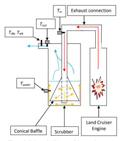
Figure 2. Schematic diagram of the transient test.
