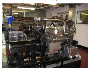
Figure 4. Engine dynamometer facility at BERF of QUT.
