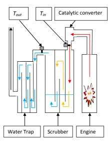
Figure 5. Schematic diagram of the steady state test of Perkins Engine.
